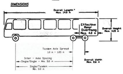
\*Note: If overall length is 12.5 m or greater, a minimum of 3 axles is required. Overall length includes bumpers.
